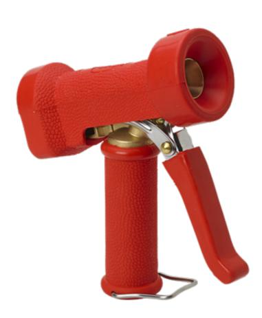
Suitable for cleaning floors and machinery including rinsing off work surfaces and walls after chemical foaming. Squeezing the rubber isulated trigger determines the jet pattern. The water jet can also be adjusted using the screw at the end of gun. The arrow on the gun shows the water spray direction. Use 0712, 1/2" or 0715, 3/4" hose nipples to be screwed into the bottom of the gun.
