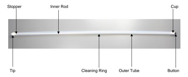
Diameter of Outer Tube: 35mm
