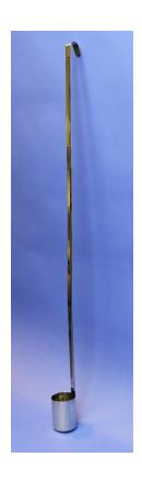
Method of Construction: Crevice free, all welds ground and polished
