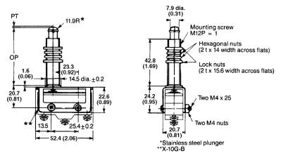
**Note:** Unless otherwise specified, a tolerance of  $\pm$  0.8 mm applies to all dimensions.
