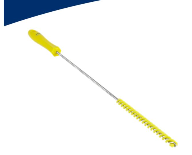
The smallest diameter of the tube cleaners is used to clean small pipes and very narrow spaces between machine parts. The filaments are attached to a twisted stainless steel rod which makes chemical resistant and strong. Example of use; sausage filler tubes.
