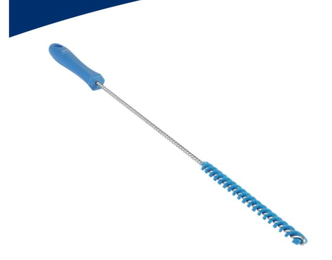
The smallest diameter of the tube cleaners is used to clean small pipes and very narrow spaces between machine parts. The filaments are attached to a twisted stainless steel rod which makes chemical resistant and strong. Example of use; sausage filler tubes.
