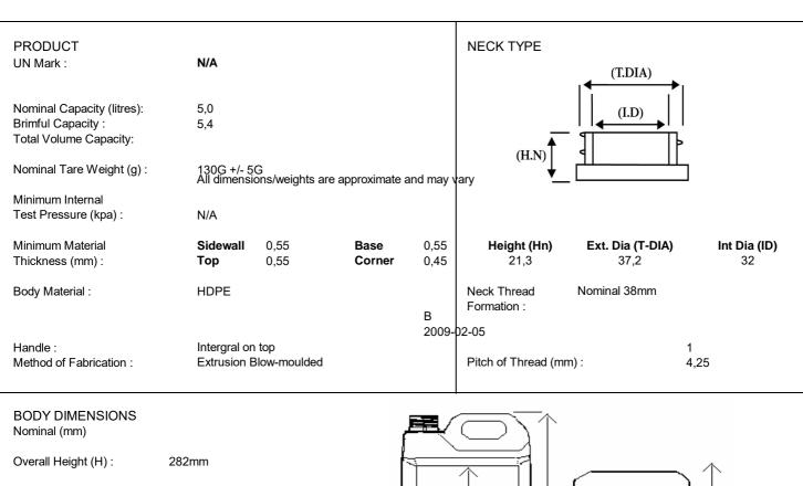
Body Section (L): 185.9mm Body Section (B): 133.6mm Label Panel width (LP): 130mm Label Panel Height (LPH): 163mm
