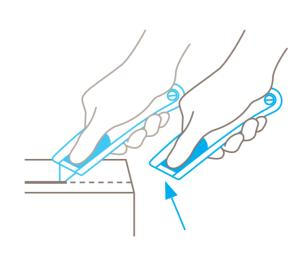
The blade automatically retracts into the handle the moment cutting ceases. Even when the slider is still **being held forwards**.
