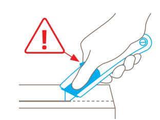
**Do not cut** when the blade-change facilitating rocking is open!
