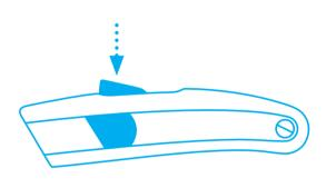
Now **rotate or change the blade** and carefully release hold of the slider. Close the rocking device.
