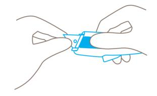
Move the slider fully forwards. Turn the handle so that the **transparent blade cover faces upwards**.
