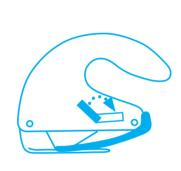
**Lift** the catch and move downwards until its end covers the blade change button.
