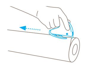
**Pierce** film and paper sheets at the required position using the point of the metal foot.
