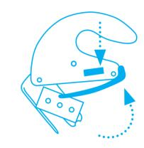
Press the catch again and insert the metal foot back into the handle until it **clicks**. Check that the foot is correctly inserted.
