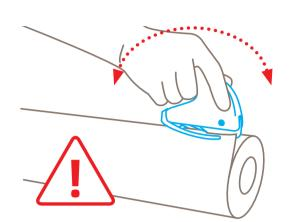
Only cut by sliding. Cutting by levering may break the metal foot.
