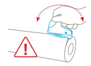
Only cut by sliding. Cutting by levering may break the metal foot.
