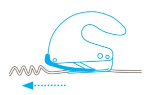
Whether cutting foam or film, the bendable plastic material-guide reliably stops material jamming in front of the blade.
